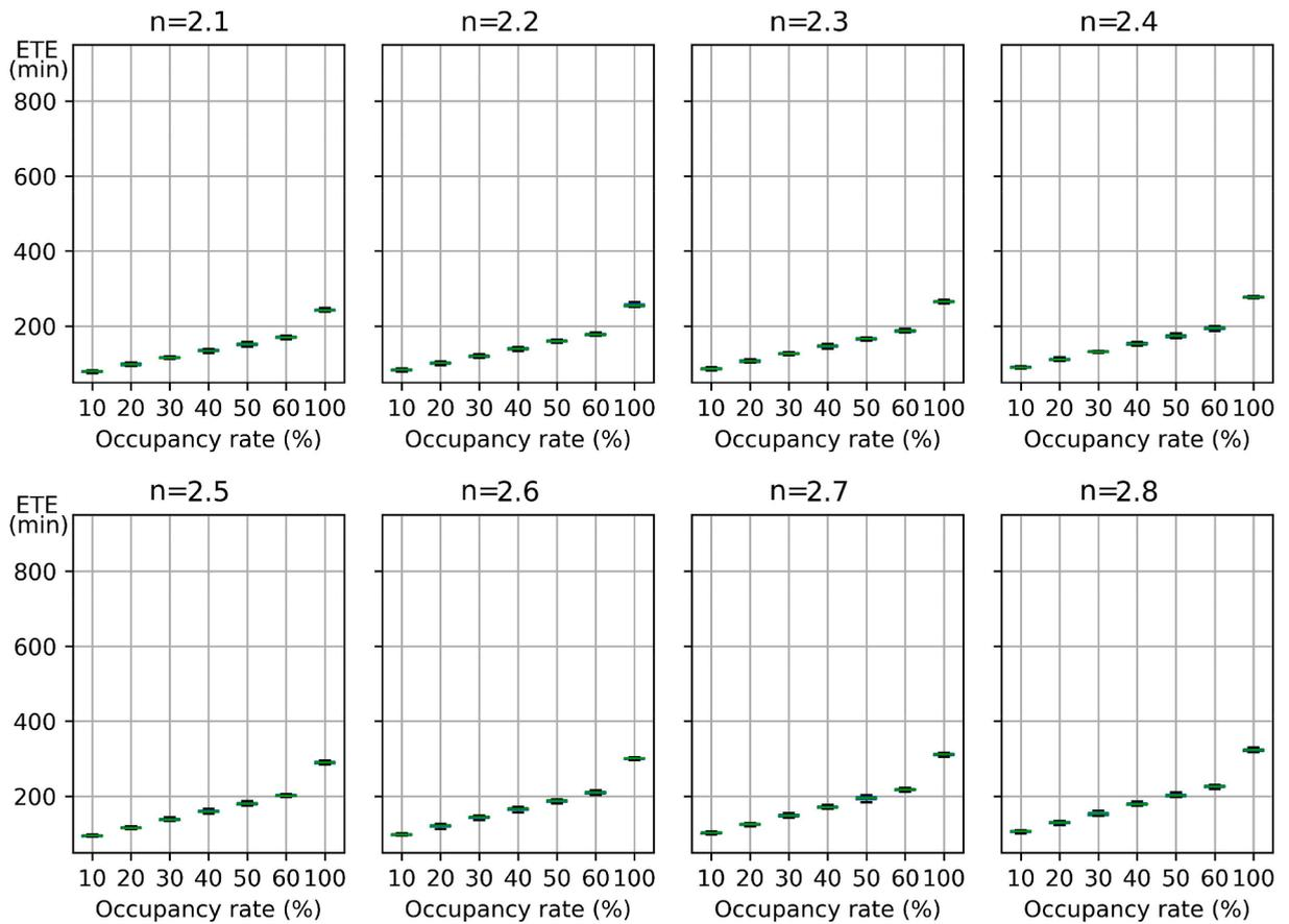
Fig. 9. The derived time needed for 50% of the vehicles to leave the risk area.
