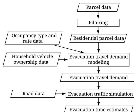
**Fig. 4.** The flowchart of the evacuation modeling procedure.
